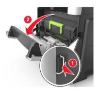
3. Pull the toner cartridge out using the handle.
